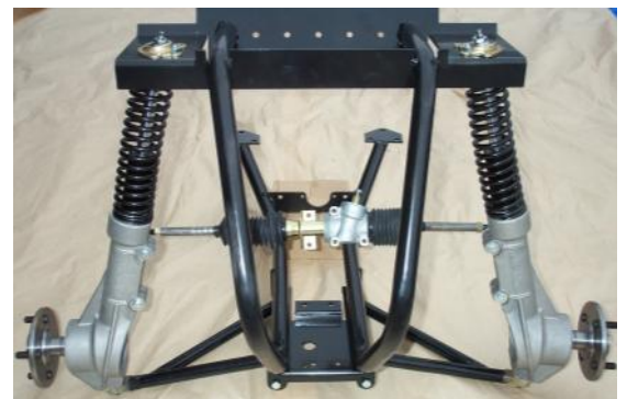
Two wheel drive kit, (optional steering rack shown)
